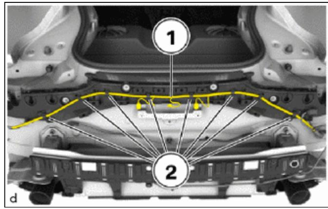
(c) Remove the nuts (1) and guide for the No. 1 rear bumper support (2).
