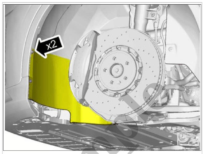
Remove the screws. Fold marked part aside.
