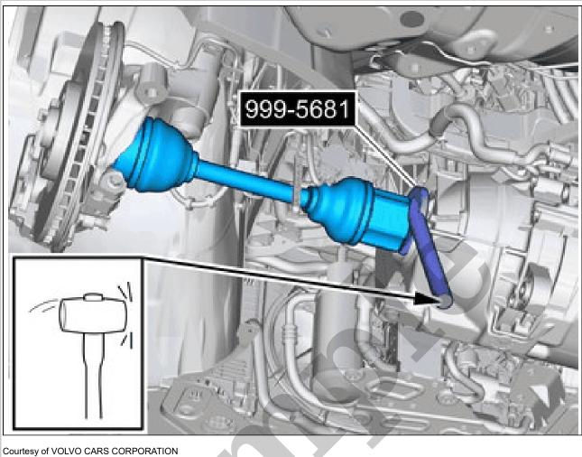
Loosen the marked detail.
