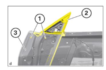
(d) Make sure the front door belt front seal (2) is correctly seated.
