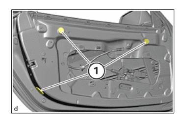
(d) Release the nuts (1) on the front door glass sub-assembly with the special tool 0 496 726 (51 0 400). While doing so, hold the
