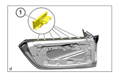
(b) Correctly position the front door glass inner weatherstrip (1) and engage in the clamps (2).
