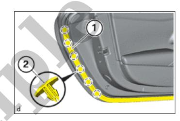
(a) Engage the clips to install the front door weatherstrip (1).
