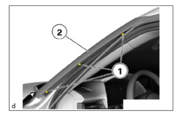
(c) Disengage the claws (1) to remove the roof drip side finish moulding (2).
