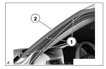
(d) Connect the front door window frame front moulding.
