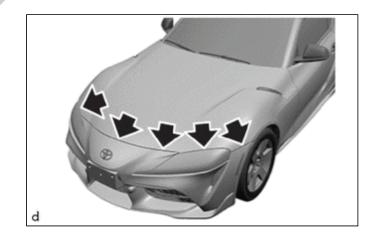
(f) Check the gap dimensions (arrows) between the hood sub-assembly and the headlight assemblies.
