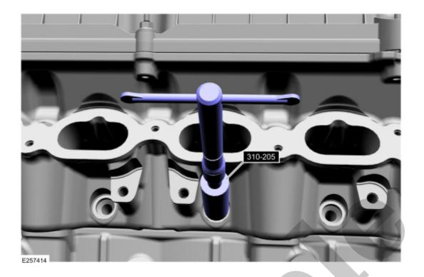
12. 1. Remove and discard the fuel injector O-ring seals.
