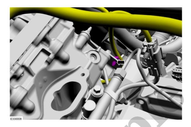
8. Disconnect the fuel injector main harness electrical connector.
