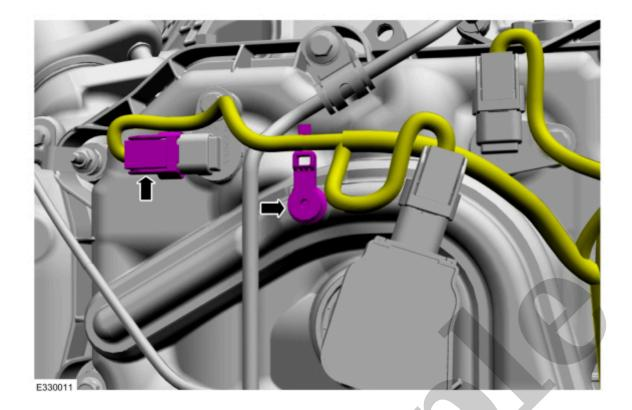
9. Install the high-pressure fuel line shield, then install and tighten the high-pressure fuel line shield retainers.
