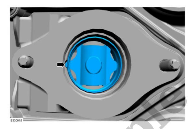
4. Install a new high-pressure fuel pump O-ring seal. Lubricate with clean engine oil.
