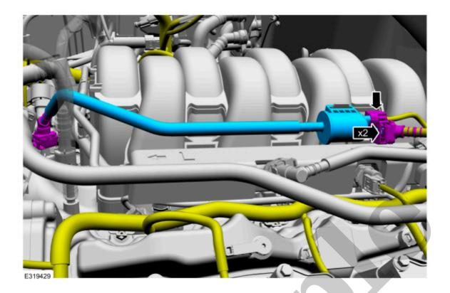
4. Disconnect the quick release couplings. Follow the directions for the quick release coupling type 1.
