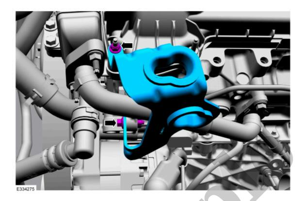
12. Remove the EGR tube retainers, then remove the EGR tube.
