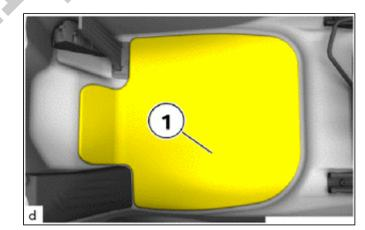
(b) Turn the No. 1 mat set plates (1) by 90° and remove upward from the front floor carpet assembly.
