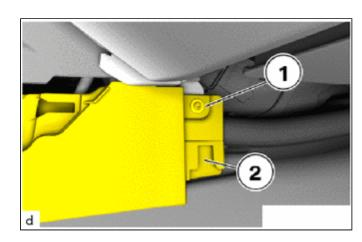
(c) Loosen T20 screws (1) on the console box assembly (2) on the front.
