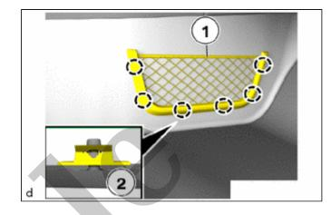
(a) Detach the clips (2) to remove the footwell storage net (1).
