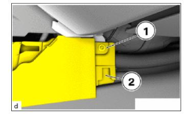
(c) Loosen T20 screws (1) on the console box assembly (2) on the front.
