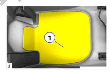
(b) Turn the No. 1 mat set plates (1) by 90° and remove upward from the front floor carpet assembly.
