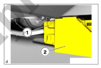
(b) Loosen T20 screw (1) on the console box assembly (2) on the right.
