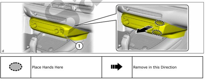
(g) Pull the instrument panel finish lower panel (1) straight forward, detach the guides (3) and the clip (2), and pull it out toward you.
