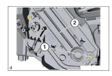
(b) Remove the heater radiator unit sub-assembly (2).
