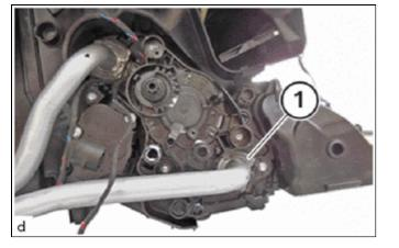
(1) Disengage retaining clip (1) using screwdriver upwards.
