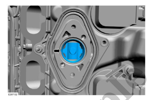
4. Inspect the high-pressure fuel pump mounting plate seal, clean and replace as needed. Lubricate the seal with clean engine oil.
