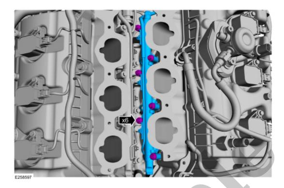
9. Disconnect the fuel injector electrical connectors.
