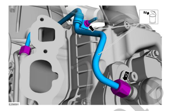
6. Release the left electrical connector retainer from the rear of the left cylinder head. Disconnect the left fuel injector main harness electrical connector.
