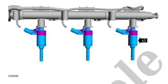
7. Remove and discard the fuel injector clips.
