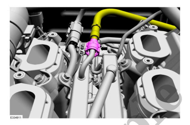
5. Disconnect the fuel rail fuel tube quick release coupling.
