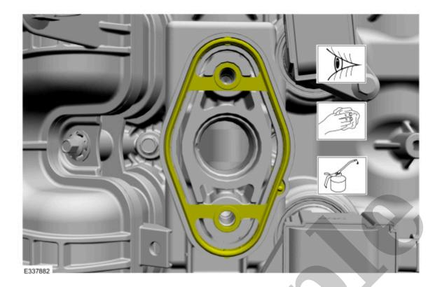
3. Apply clean engine oil to the high-pressure fuel pump mounting pedestal bore, the drive lobe and all of the roller tappet.
