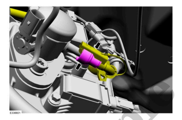
9. Connect the high-pressure fuel pump electrical connector.
