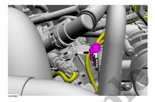
5. Install the charge air cooler outlet pipe, then tighten the charge air cooler outlet pipe clamp.
