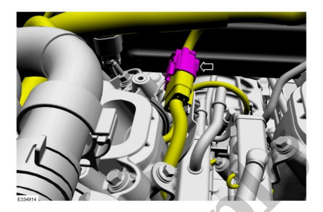
6. Connect the fuel rail fuel tube quick release coupling.
