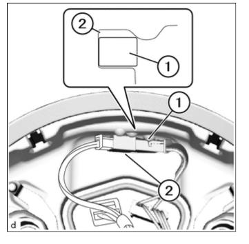
(d) Apply even amounts of pressure and press the horn button assembly (1) into the steering wheel assembly until the airbag unit audibly and noticeably engages.
