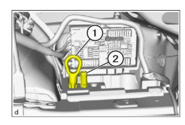
(b) Detach the claws (2) to remove the rear power distribution box (1).
