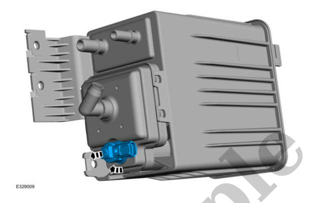
3. Release the tabs and remove EVAP (evaporative emission) canister ventilation filter.
