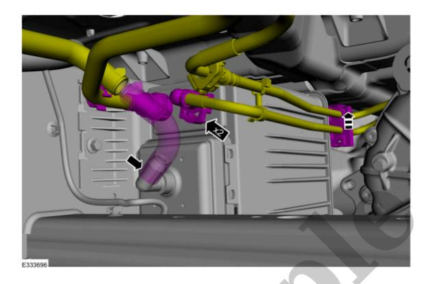
4. Detach the fuel line routing clip from the EVAP (evaporative emission) canister and position the line aside.
