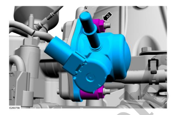
15. Remove and discard the high-pressure fuel pump O-ring seal.
