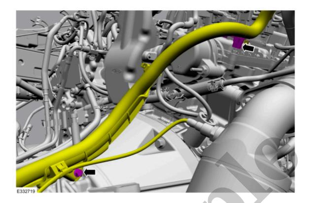
6. Detach the wiring harness retainers.
