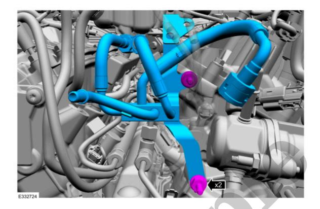
12. Disconnect the high-pressure fuel pump electrical connector.
