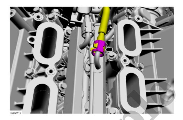
6. Attach the fuel rail harness retainer.
