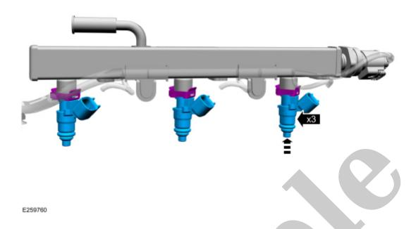
3. Connect the fuel injector electrical connectors,
