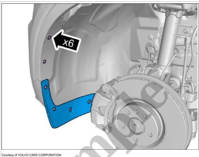
Remove the screws. Remove the marked part.
