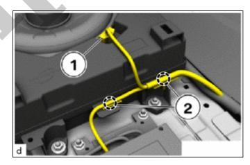
(a) Unlock plug connection (1) and disconnect.
