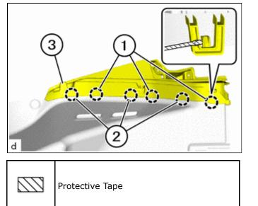
(b) Detach the guides (2) to remove the deck side trim cover LH (3) from the deck trim side board LH.
