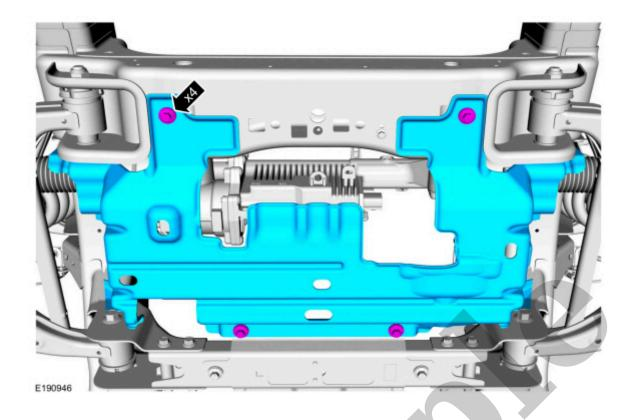
5. If equipped, install the skid plate and bolts.
