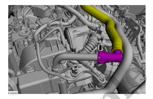
10. Loosen the clamps and disconnect the differential pressure sensor hoses.
