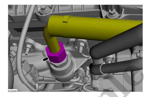
13. Remove the EGR (exhaust gas recirculation) assembly.
