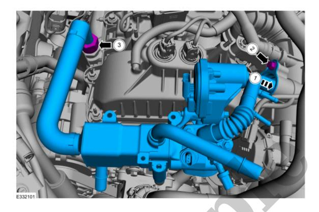
5. Install the EGR (exhaust gas recirculation) cooler fasteners and hand tighten at this stage.
