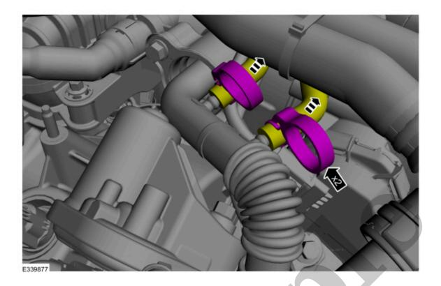
9. Remove the EGR (exhaust gas recirculation) inlet tube nut.
