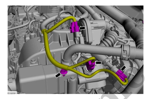
6. Disconnect the lower coolant hose from the EGR (exhaust gas recirculation) cooler assembly.
