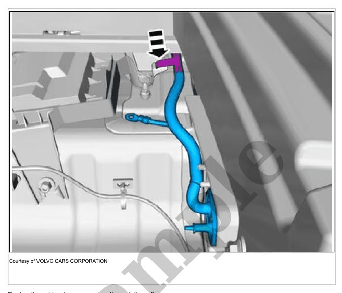
Fasten the wiring harness using the existing clips.
