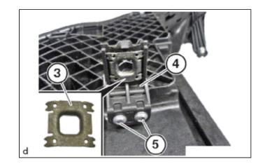
(g) Secure the new retaining ring with enclosed screws (5).
