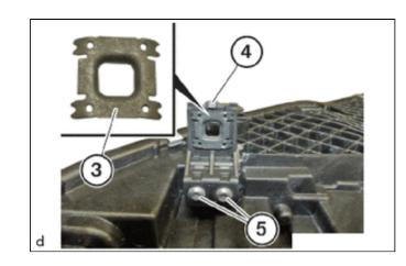
(d) Secure the new retaining ring with enclosed screws (5).
