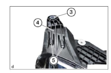
(m) Secure the new retaining ring with enclosed screws (5).
