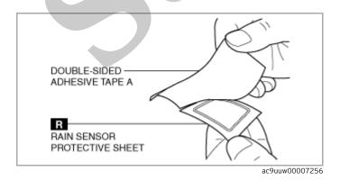
3. Adhere a new rain sensor protective sheet to the rain sensor lens.
