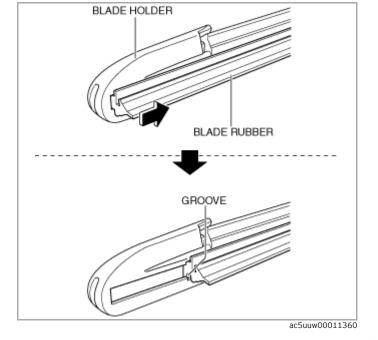
3. Pull the end of the blade rubber from the blade holder groove in the direction of the arrow and remove the blade rubber from the blade holder.
