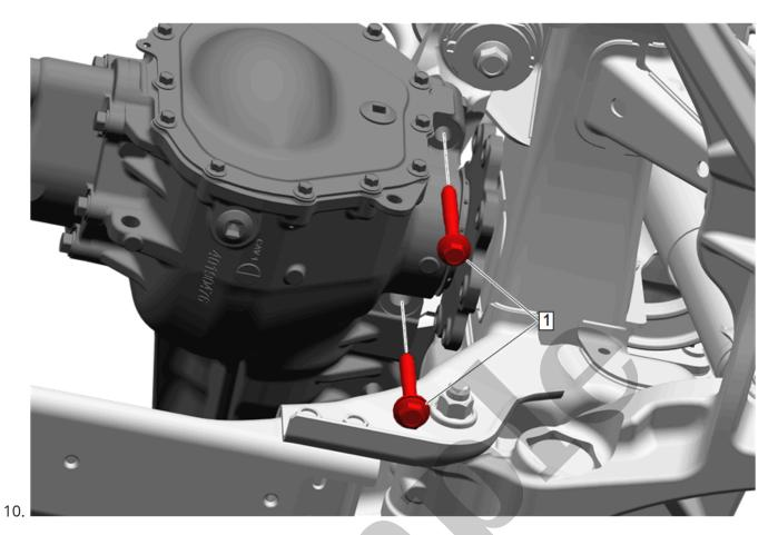
Front Differential Carrier Bolt(1) »Remove[2x]
