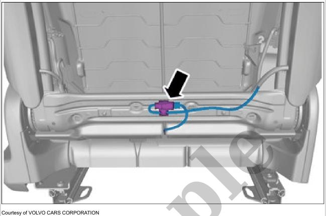
Remove the cable harness clips. Remove the marked part.
