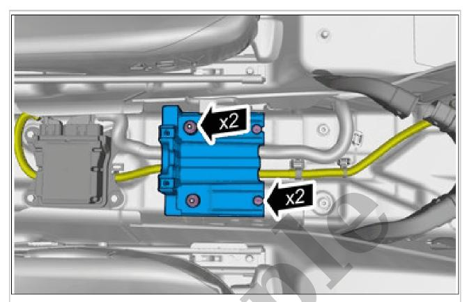
Remove the screws. Torque: M6, 10Nm Loosen the clips. Remove the marked part.
