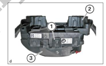
(c) Remove the spiral cable sub-assembly (3) from the turn signal switch assembly (2).
