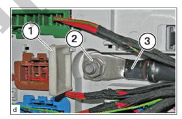
(b) Install the positive battery cable (3).
