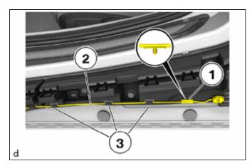
(b) Disconnect the floor wire (2) from holders (3).
