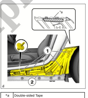
(g) Install the No. 4 body outside moulding pad (2) with the clips (1).
