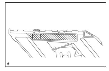
(f) Remove the release paper from the 20 mm (0.787 in.) double-sided tape.
