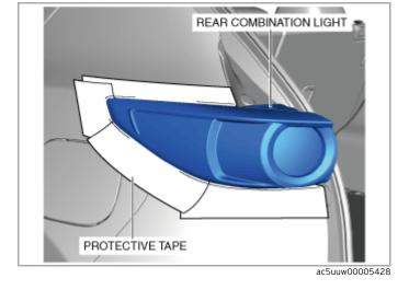
7.Pull the rear combination light in the direction of arrow (1) shown in the figure and pull out the rear combination light from the body.
