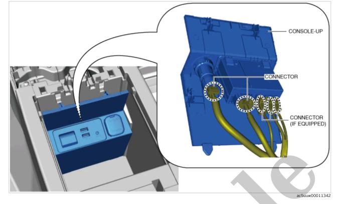
6. Move the console-up in the direction of the arrow shown in the figure, detach the guides from the rear console, and remove the console-up.
