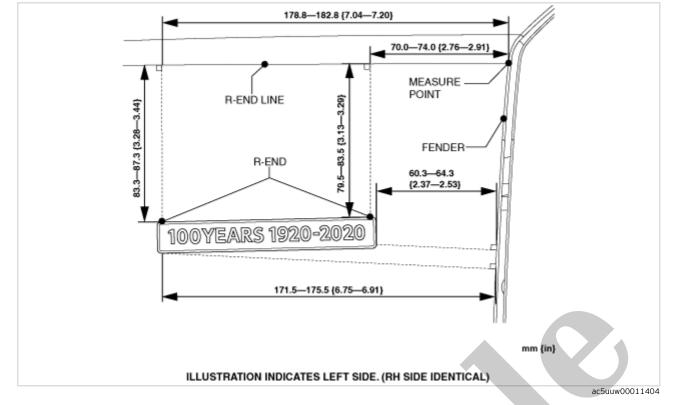
4.Press the ornament with the force of 29.4 N (3.0 kgf, 6.61 lbf) to adhere the double-sided adhesive tape to the ornament installation area.
