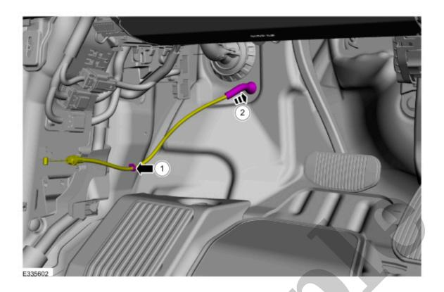
4. Route the hood latch release cable through the engine compartment.
