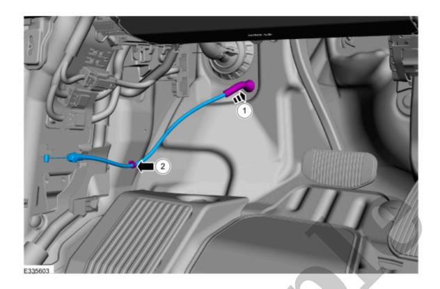
2. Route the hood latch release cable through the engine compartment.
