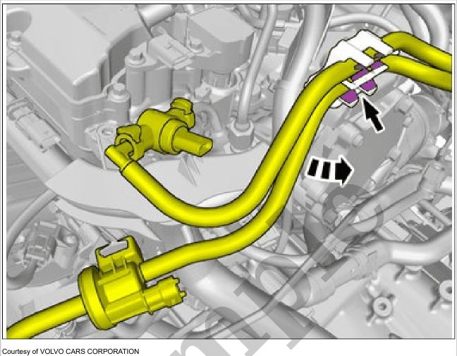
Release the catches. Loosen the marked detail. Fold marked part aside.
