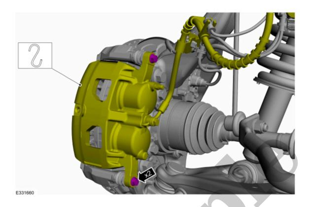
4. Remove the brake pads.
