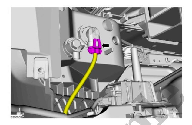
4. Rotate the fog lamp bulb counter clock-wise and remove the bulb.
