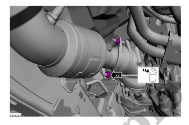
5. Loosen the clamp and remove the LH (left-hand) catalytic converter.
