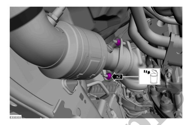
5. Loosen the clamp and remove the LH (left-hand) catalytic converter.
