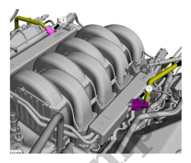
6. Remove the fuel rail insulators.
