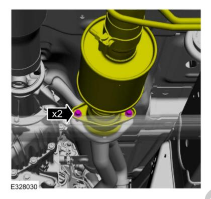
12. Install the heat shield and bolts.
